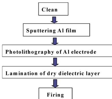
FIGURE 3 — Fabrication process of the substrate.
