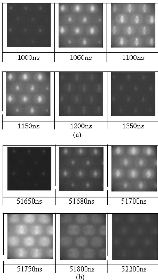
FIGURE 10 — Sustain discharge process photographed by an ICCD. (a) Positive sustain pulse on scan electrodes. (b) Negative sustain pulse on scan electrodes.
