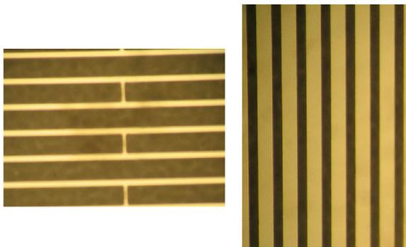
FIGURE 6 — High-quality Al-electrode pattern for bus/date electrode.
