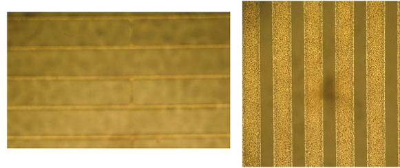
FIGURE 7 — Dielectric layer made of dry film on the front/rear substrates.
