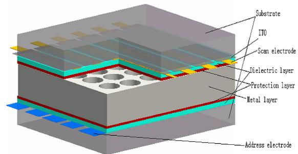
FIGURE 1 — Panel structure of the SMPDP.
