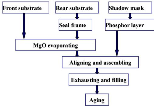
FIGURE 2 — Fabrication process of 25-in. SVA SMPDP.
