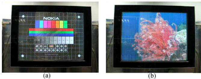
**FIGURE 11** — Images displayed on a 25-in. SVGA SMPDP. (a) Standard test pattern. (b) Video image.
