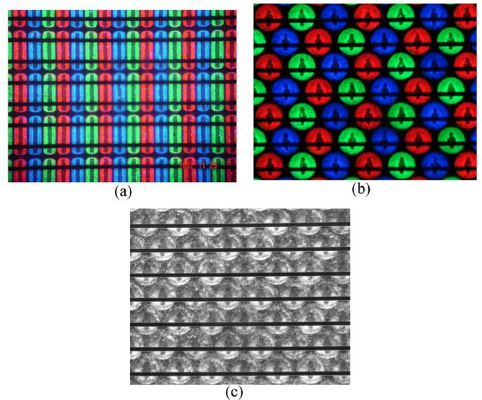
FIGURE 8 — Comparison between rectangular- and round-type subpixels in an SMPDP. Comparison between phosphor and discharge. (a) Rectangular subpixel, (b) round subpixels, and (c) phosphor layer before discharge of (b).
