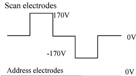
FIGURE 9 — Sustain pulse waveform on the electrodes.
