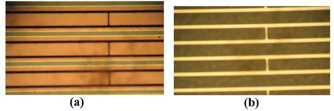
FIGURE 4 — Bus electrode in the front substrate. (a) With ITO, (b) without ITO.
