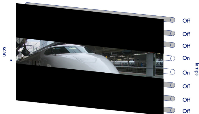
FIGURE 7 — A scanning backlight is a direct-lit backlight, in which the light sources emit light only for a short fraction of the frame-period time, and in which the light sources are ignited one after the other.
