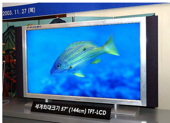
FIGURE 12 — The world's largest TFT-LCD (57 in.) with full HD (1920 × 1080) resolution using S-PVA mode.
