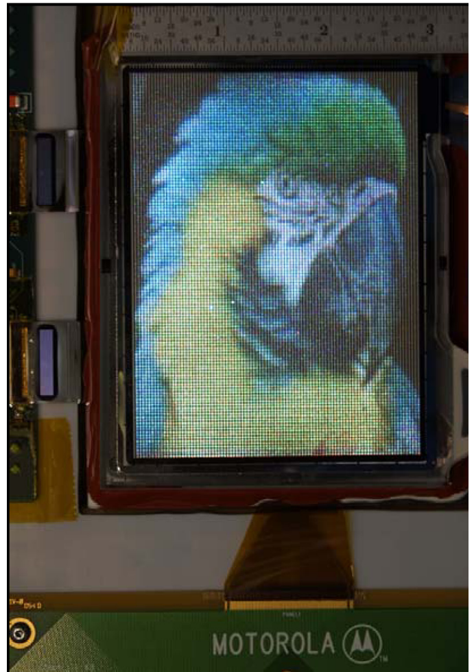
FIGURE 9 — Packaged 4.6-in.-diagonal NED (0.726-mm pixel) showing a color video image of a parrot.
