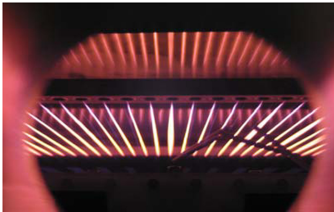
FIGURE 4 — Array of filaments at growth temperature in an HF-CVD system.
