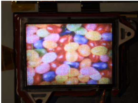
FIGURE 10 — Two color images on NED demonstrators depicting the excellent color gamut representative of CRT (P22) phosphors.
